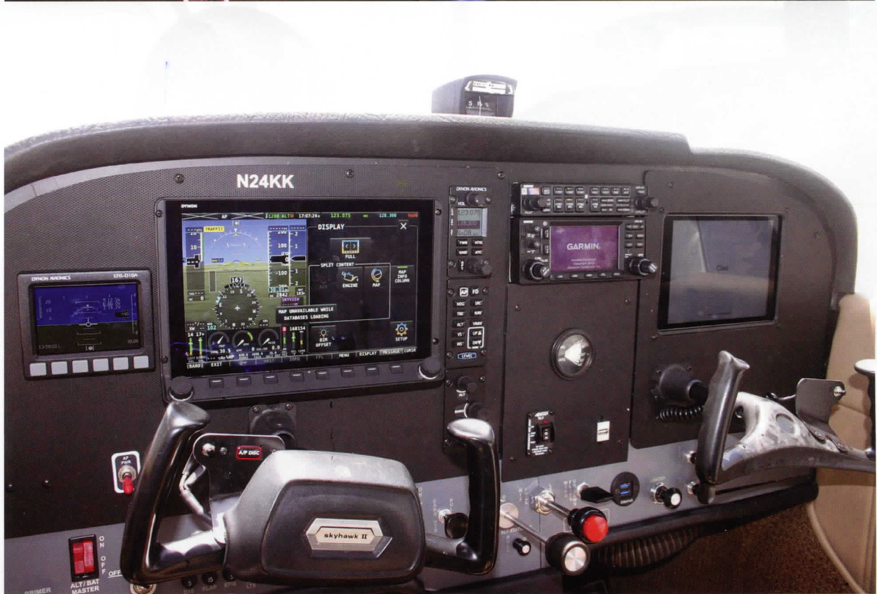
N24KK's panel features 21 st -century avionics from Dynon, coupled with a Garmin GNS 430 navcom. A panel-mount Apple iPad can be added for monitoring traffic and weather.
